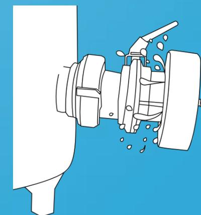
Guiding the cleaning liquid around the plug's nose
